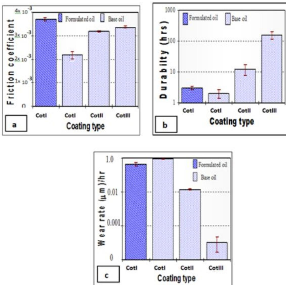
Fig 2 - (a) Friction coefficient data; (b) Mean durability of coated rollers at 1540 MPa; and (c) Mean wear rate / running time for steel counterface washers against various coated rollers.
