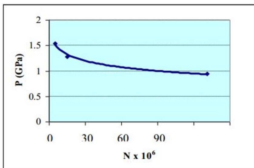
Fig 3 The relationship between the Hertzian pressure (P) and the no.
