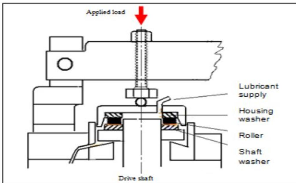
**Fig 1 Main components of the test rig head**
